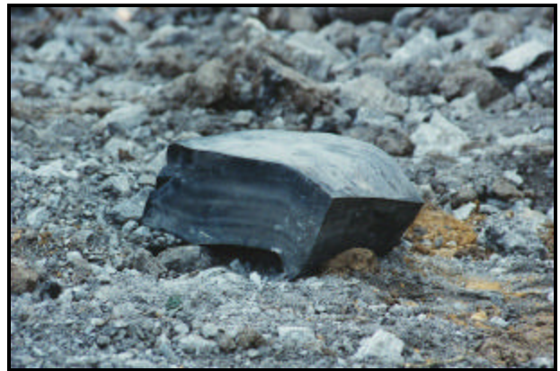
FIGURE 3.39 View of a failed elastomeric bearing pad after Izmit EQ 1999 (10)
