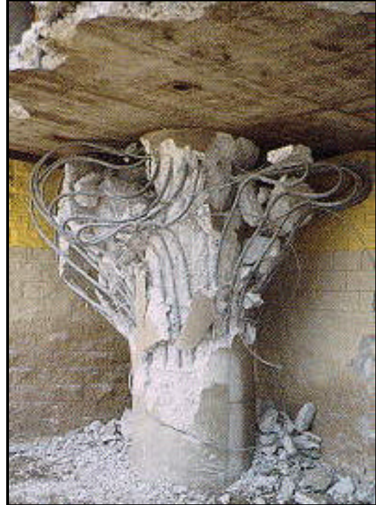
FIGURE 3.24 Failure of RC e column (11)
